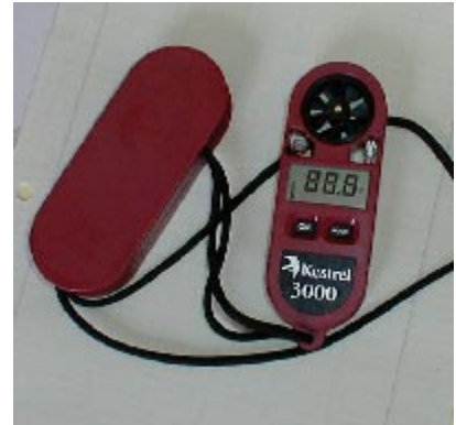
Your instrument of choice for this exercise is the Kestrel 3000 Weather Meter.
