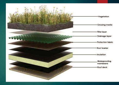
Green roof will capture and additional 18,700 gallons of storm water (roof surface 40'x20') = 800 sqft x (36" of rain annually/12" per ft) = 2400 x 7.82 gallons per cubic ft
