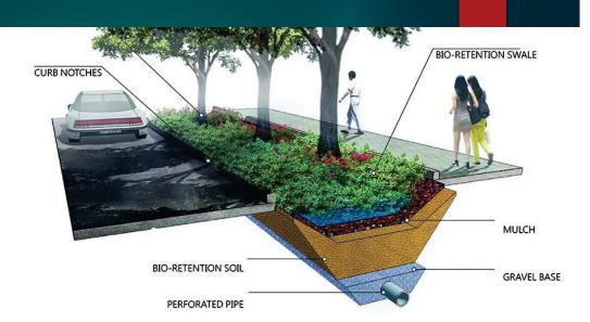
Bioswale will divert 987,000 gallons of runoff annually (road surface 200°x22') = 4400 sqft x (36° of rain annually/12° per ft) = 132000x7.82 gallons per cubic ft
