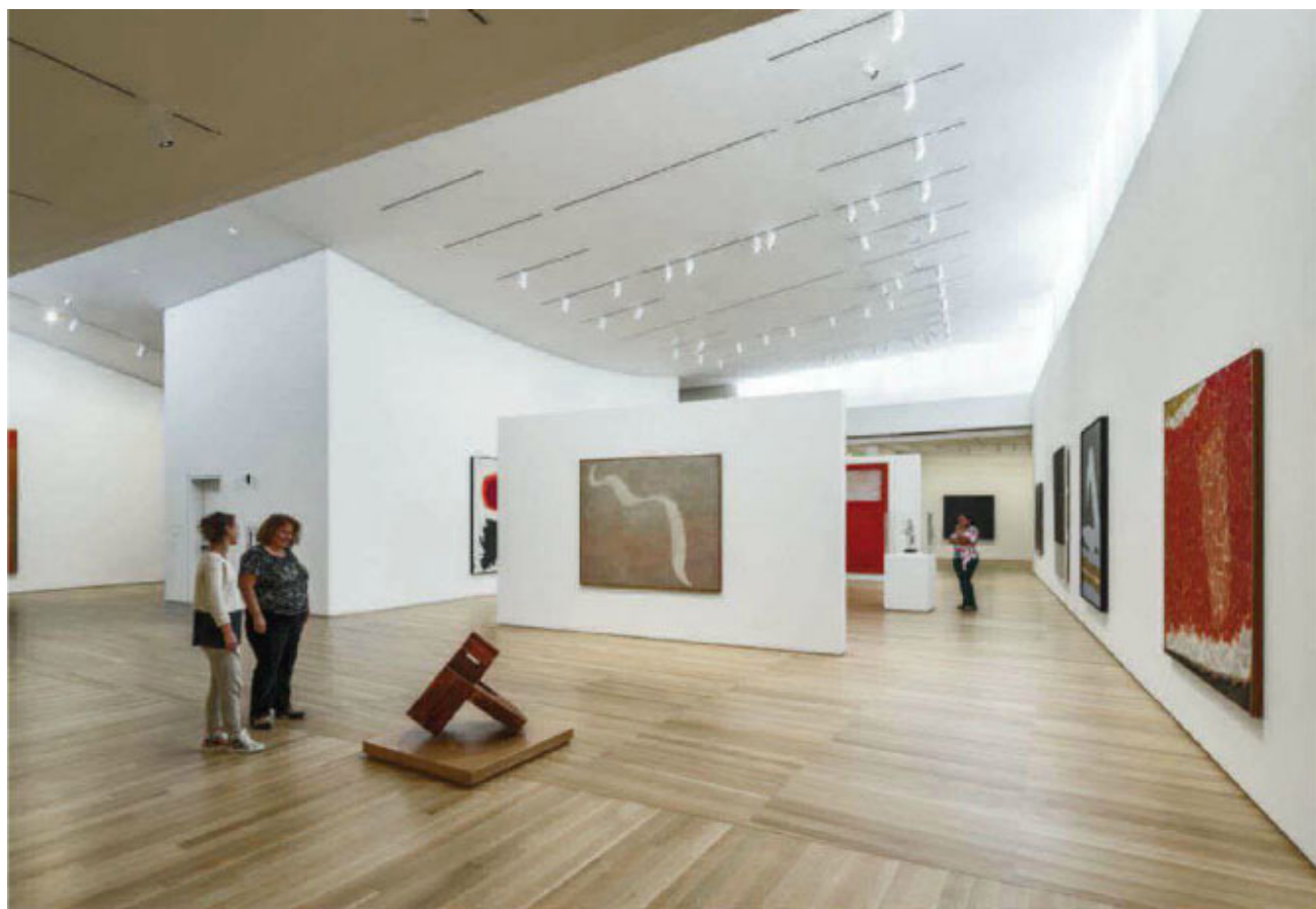
Inside the west gallery looking south, one of the three daylighted galleries, illuminated mainly by the clerestory windows. The exterior wall is to the right in this photo.
