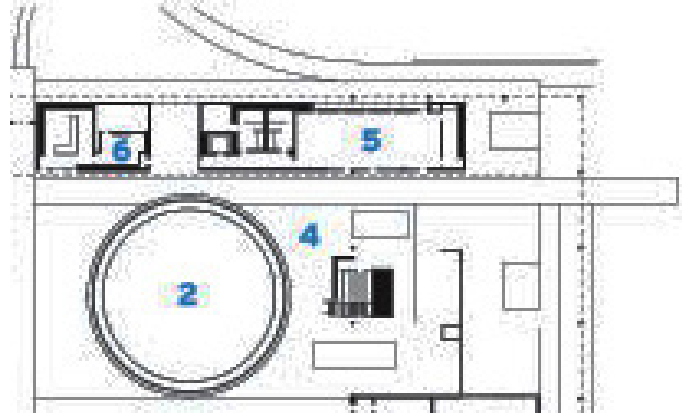
Ground floor plan. Tours and presentations for visitors start in the conference room (5) and they have access to the bathrooms between it and the control room (6).
