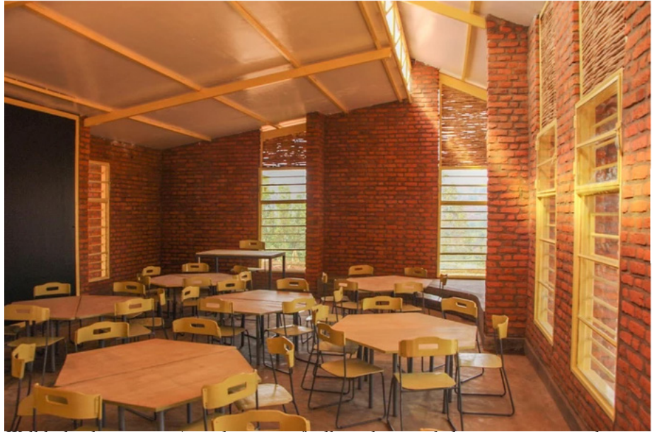
Well lit interiors. A combination of tall windows and clerestories ensure that classrooms are flooded with natural light.
