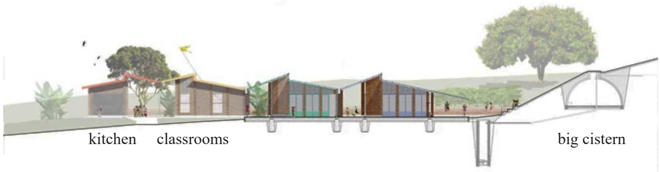
Site section showing small and big cisterns.
