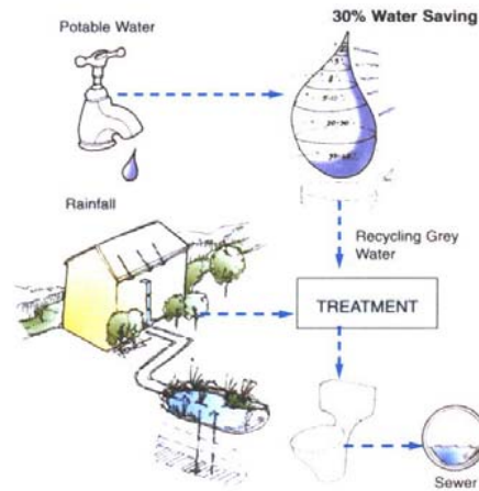
Concept Drawing of Gray Water Recycling
