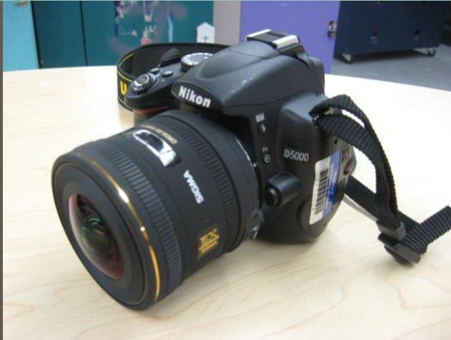
Sigma 4.5mm f/2.8 EX DC HSM circular fisheye lens mounted on a Nikon D-5000 Digital SLR camera
