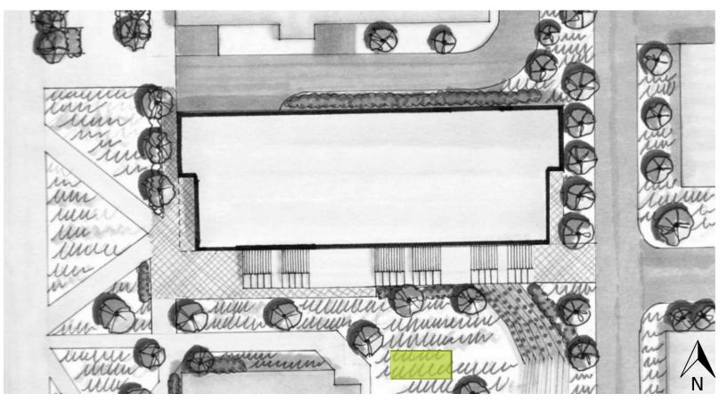
Bioswale allows for excess storm-water drainage on site
