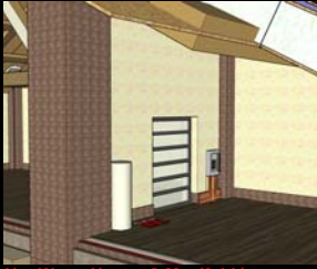
Hot Water Heater & Manifold in Mechanical/Storage Room
