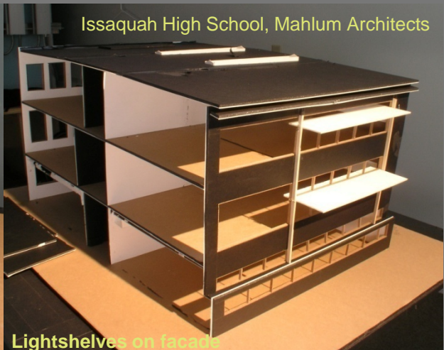
Lightshelves on facade
