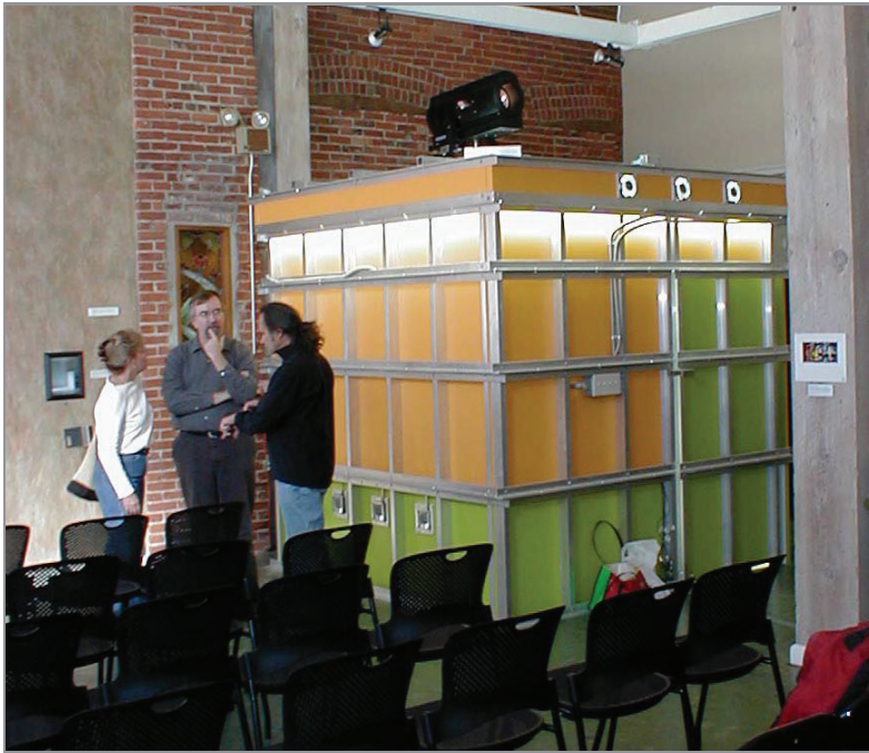
Mirror-Box Artificial Sky at IDL, Boise, ID uses twenty-two 59-watt fluorescent lamps (1,298 watts total)
