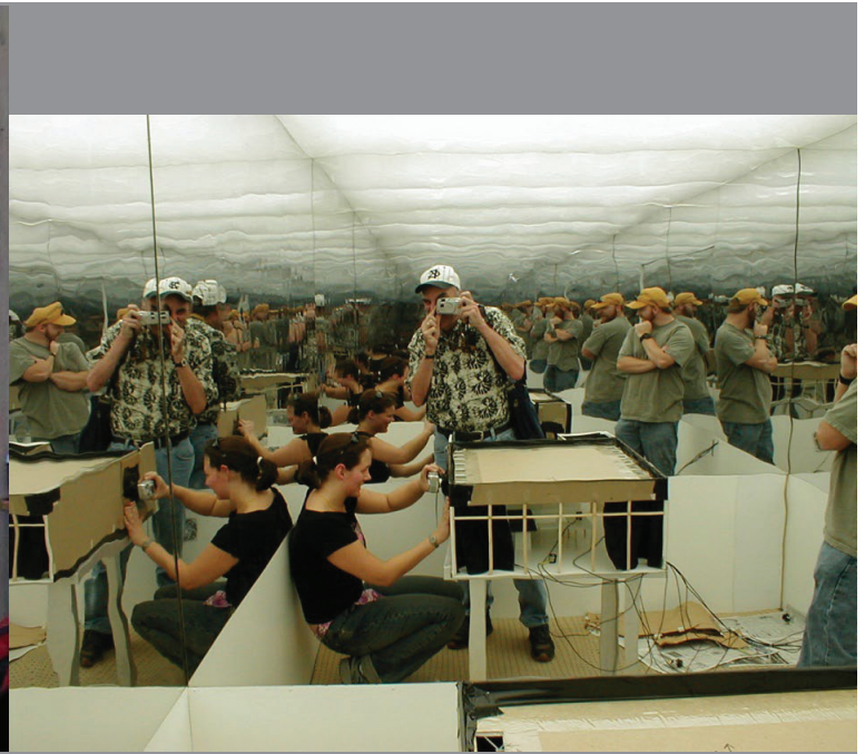
Mirror-Box Artificial Sky at IDL, Boise, ID uses twenty-two 59-watt fluorescent lamps (1,298 watts total)
