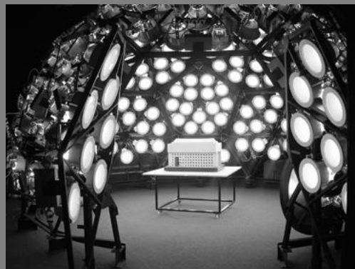
Cardiff Sky 8m diameter: 640 luminaires (20-watt Philips CL 4500K) CFLs (12,800 watts total) Bartlett Sky 5.2m diameter: 270 CFLs (5,400 watts total)
