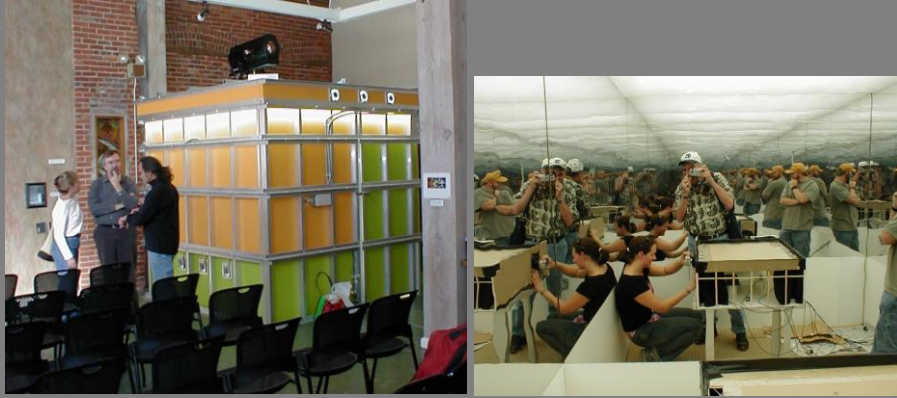
Mirror-Box Artificial Sky at IDL, Boise, ID uses twenty-two 59-watt fluorescent lamps (1,298 watts total)
