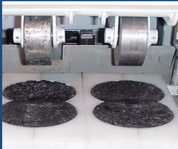
Chamber View with Hamburg Wheels and Molds
