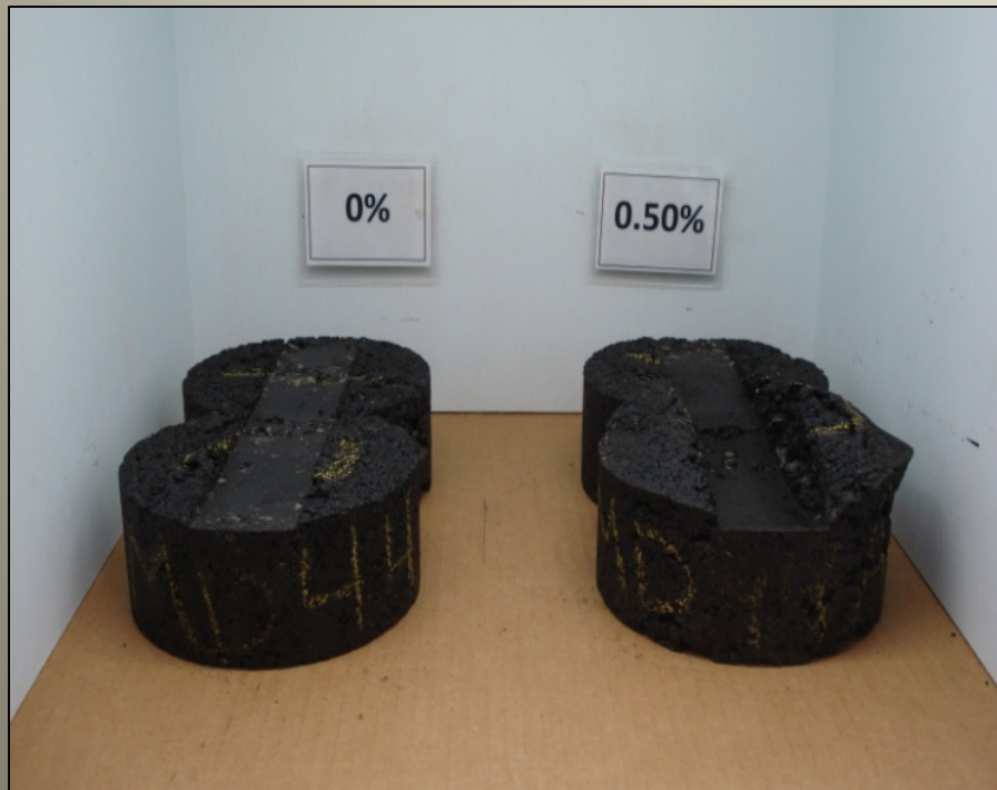
Hamburg Samples with PG64-28 “Original Formulation”
