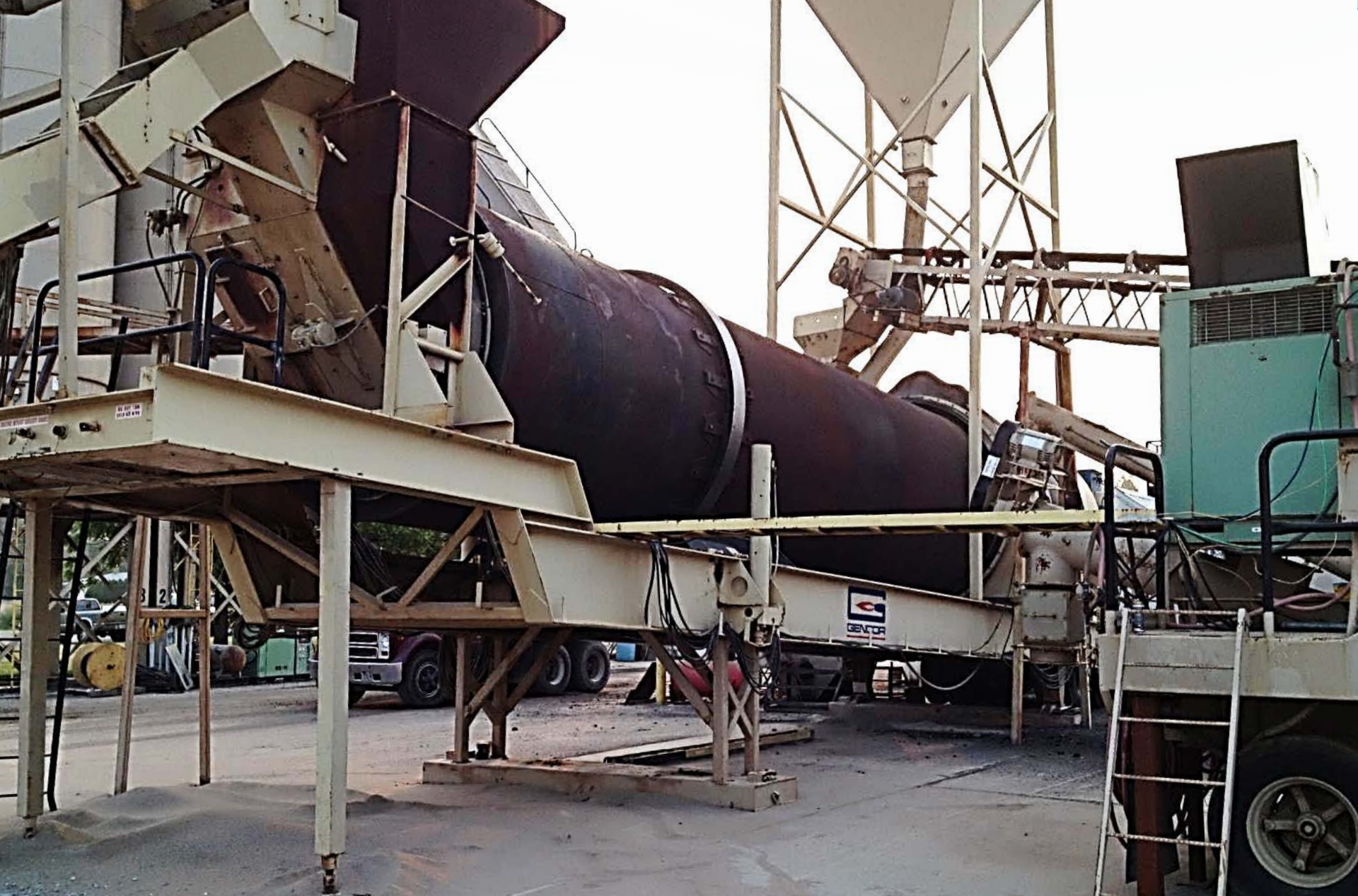
Counter-Flow Drum Mix Plant
