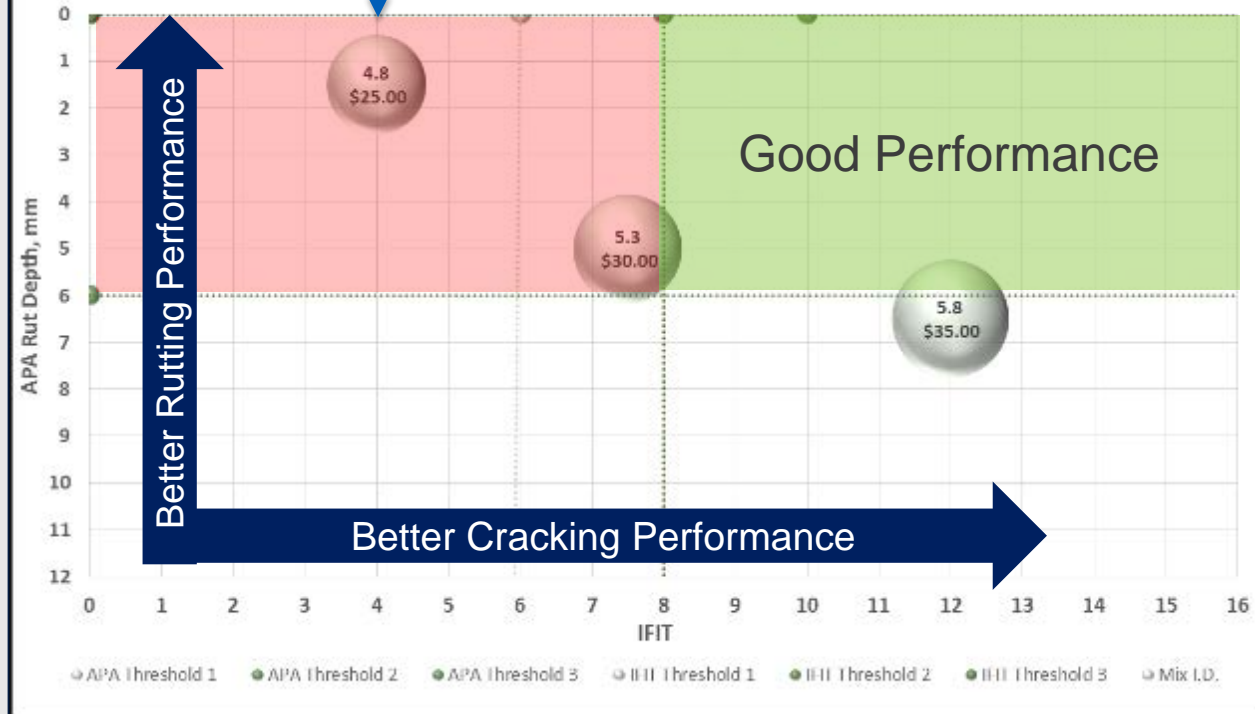
MIXTURE PERFORMANCE SPACE DIAGRAM : APA vs IFIT
