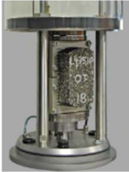
Texas Overlay Test
