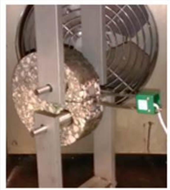
Disk Shaped Compact Tension (DCT)
