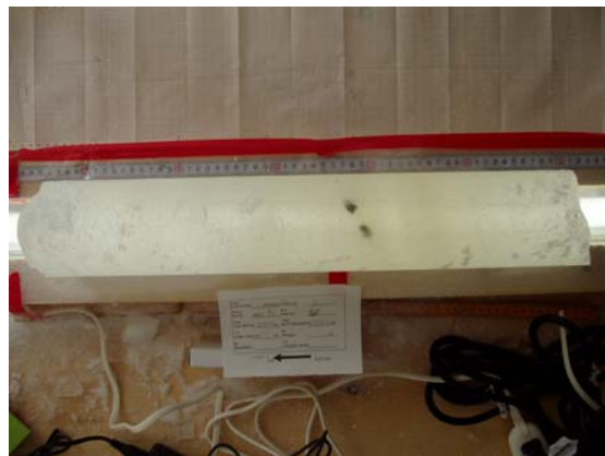
Figure 12. Loosed stones close to the bottom at 169.6 m depth.
