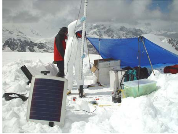
Figure 8. 'Mini-Felix' sun powered electro-mechanical drill. Zuoqiupu Glacier, 6,120 m a.s.l proposed deep drilling site. Photo by V. Aizen
