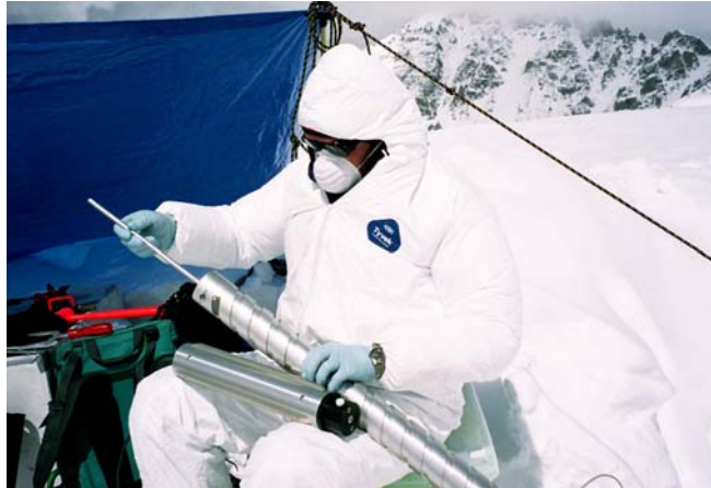
Figure 6. 'Mini-Felix' sun powered electro-mechanical drill. Drill barrel cleaning after each run. Zuoqiupu Glacier, 6,120 m a.s.l proposed deep drilling site. Photo by V. Aizen
