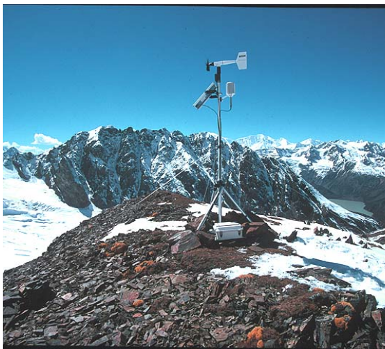
Figure 7. 'Campbell Scientific' automatic weather station established at 5,800 m, 2 km northeast from proposed drilling site at Zuoqiupu Glacier snow-firn area. Photo by D. Joswiak
