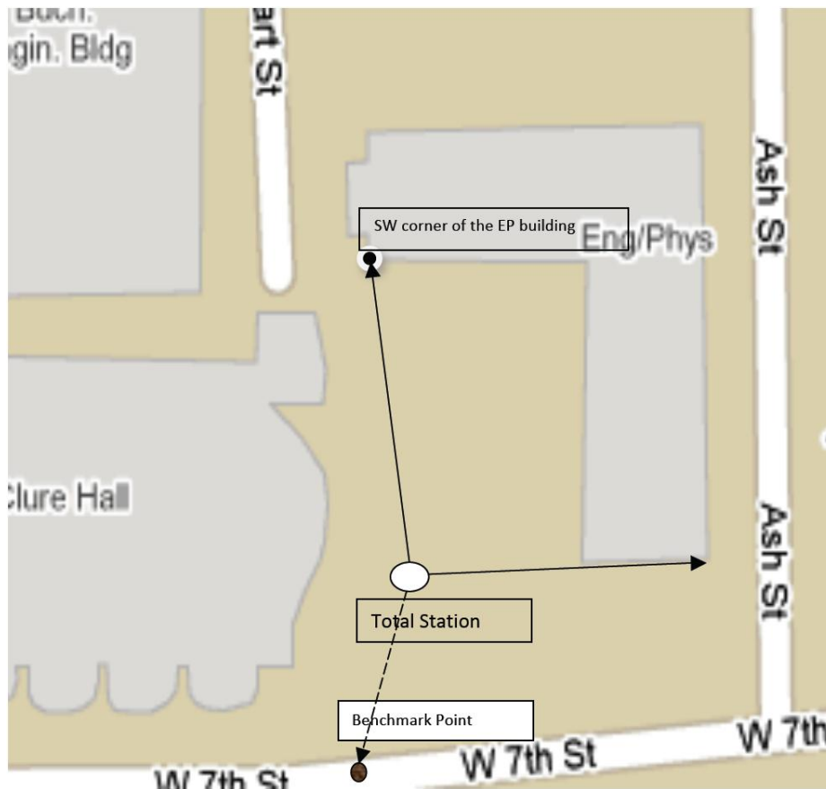
Figure 1: Engineering Physics (EP) building lawn area with points for horizontal and vertical angle measurements
