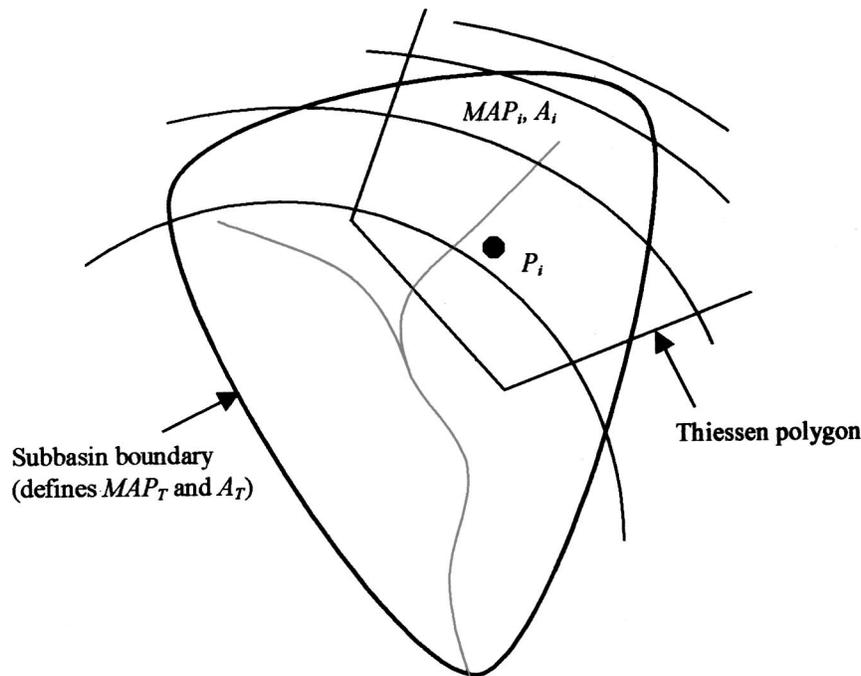
**Fig. 1.** Hypothetical subbasin with one gauging station and associated Thiessen polygon defined. Curved lines in upper right portion of figure represent isohyets.  $P_i$  = mean precipitation measured at gauging station, and  $MAP_i$  = mean areal precipitation in  $A_i$  (area defined by intersection of Thiessen polygon and subbasin boundary) as defined by isohyets.  $MAP_T$  and  $A_T$  = mean areal precipitation computed over entire subbasin and total subbasin area, respectively.
