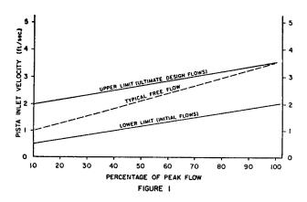
2 FPS (0.6 m/sec) is required to wash any grit that may have accumulated in the inlet flume at the lower flows into the grit chamber for removal.
