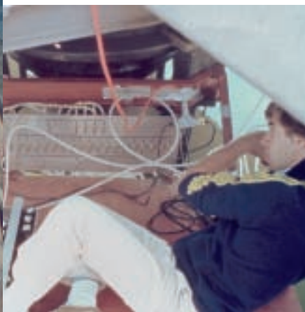
Installation of sample probes in header.
