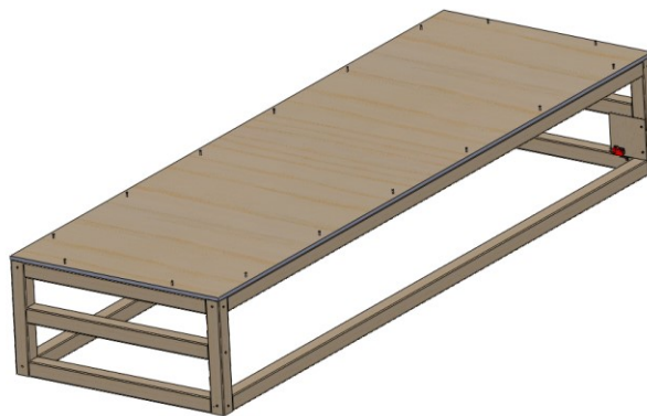
Figure 10: Flip the frame and screw the bottom panel with shiny side inside
