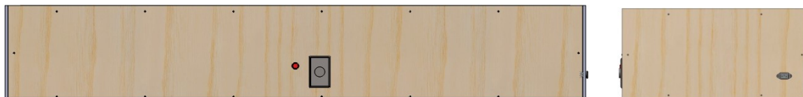
Figure 13: Secure pilot lamp and timer switch on front panel, AC power entry model on side panel
