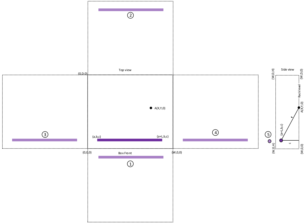
Figure 26: Reflection of the UV lamp from aluminum foil. Reflection with only one bounce of UV ray is shown here. Higher order of reflections are neglected.
