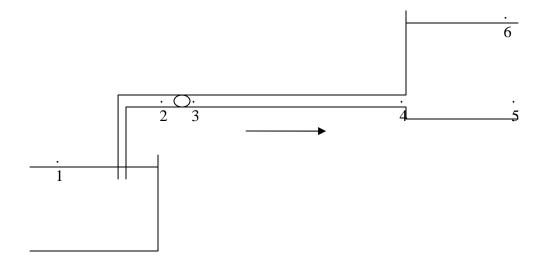
Water is pumped from the reservoir on the left to the reservoir on the right. The pump located between points 2 and 3 sits 4 m above the water surface of the left reservoir, and 2 m below the water surface of the right reservoir. The pipe diameter is 10 cm along the entire length of the pipe. The length of the pipe on the upstream (suction) side of the pump is 20 m, and the length on the downstream side is 80 m. The pump provides 8.7 m head. Friction headloss can be
