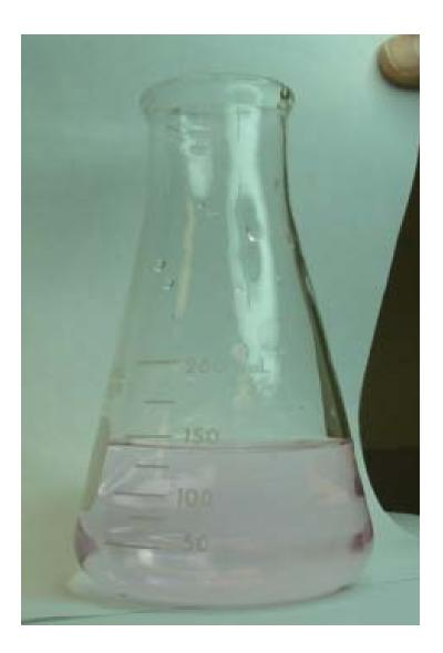
In Experiment 3, phenolpthalein is used as an indicator for the titration of a KHP solution with 0.1 M NaOH.
