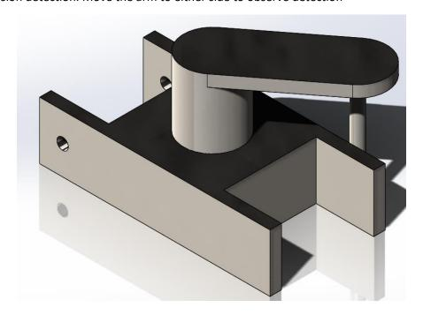
3&4. Insert the part "rod" into the assembly and create the mates shown below. Insert "bushing" into the assembly. Apply the mates shown below. What is the center of mass of the assembly with respect to coordinate system 1?
