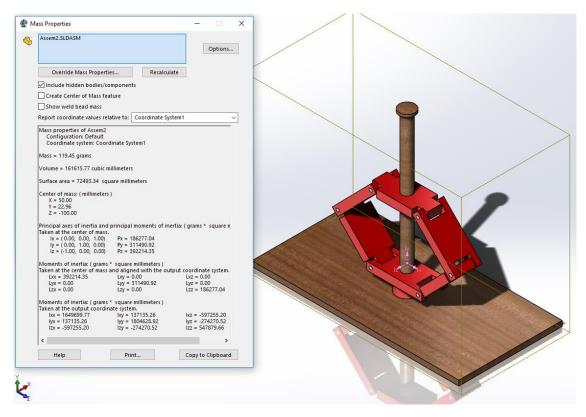
9&10. Replace "base" with "base2". What is the center of mass of the assembly with respect to Origin1?
