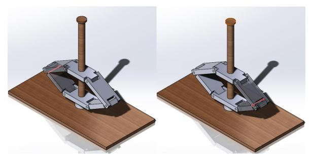
6&7. Change the last mate from 55 to 75mm. Create the coordinate system shown below.
