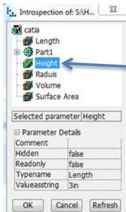
Select the desired parameter to attach to the input/output from the design tree.
