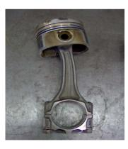
Pictured is a bent connecting rod, this is an example of the strength and endurance for which ARP connecting rod bolts are designed.
