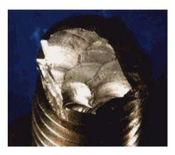
This bolt displays microvoid coalescence which is attributed to interfacial cracking between inclusions and the surrounding material matrix. This is usually a high energy process that occurs at high crack growth rates.
