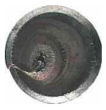
This bolt is a good display of the noticeable difference between the fatigue crack surface and the final fracture surface. Also notice that the crack started on the inside of the bolt and propagated toward the surface until final fracture occurred.
