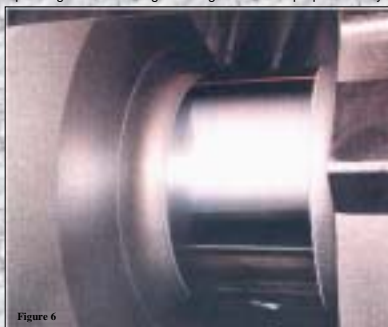
Figure 6 (Figure 6) Crankshaft fatigue life is increased by shot peening the radii on the shafts journals.
