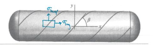
Pressure tank shown above is fabricated from spirally wrapped metal plates with an orientation of  $\beta = 40^{\circ}$ . The ID of the tank is 720 mm, and wall thickness is 8 mm. If the gage pressure inside the tank is 2.15 MPa, calculate:
