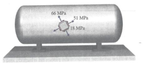
Pressure tank shown above is has stress state as shown. The ID of the tank is 830 mm, and wall thickness is 10 mm. Calculate the gage pressure inside the
