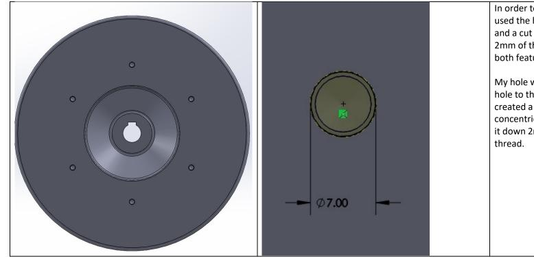
In order to create the M7 hole pattern I used the hole wizard to make one hole and a cut extrude to remove the first 2mm of thread then circular patterned both features.
