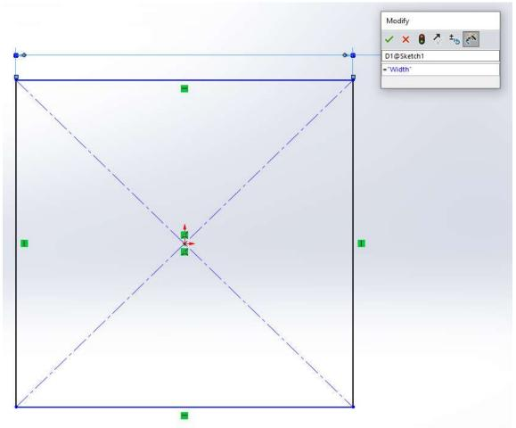
You can check that the dimension is linked to the variable if it has  $\Sigma$  in front of the dimension, like this:
