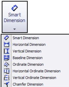
Baseline dimensioning references the dimension from a single edge or vertex. Ordinate dimensioning reference a chosen zero point (edge, point, vertices, or arc) and the selected starting point is denoted with a zero. A chamfer dimension accurately dimensions a chamfer.
