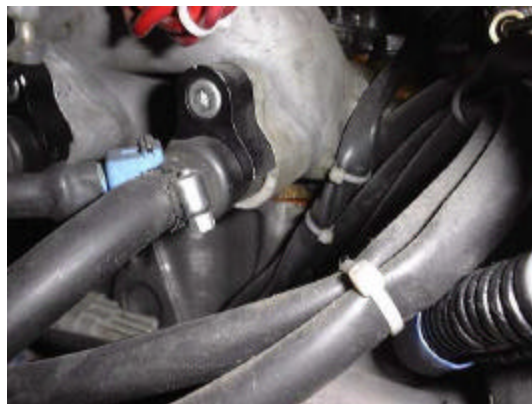
Figure 6. Yanmar diesel engine intake manifold, fuel injectors (left side).
