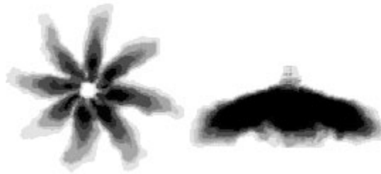
Figure 2. Flame pattern exiting the nozzle of the catalytic igniter
