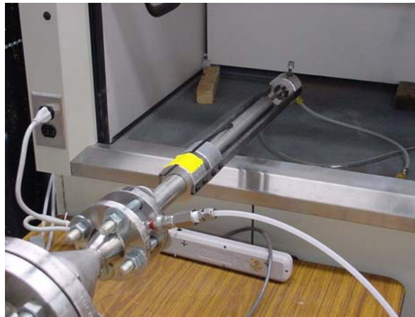
Figure 4. Indexer inserted into the reaction section to locate repeatable axial locations for gas sampling
