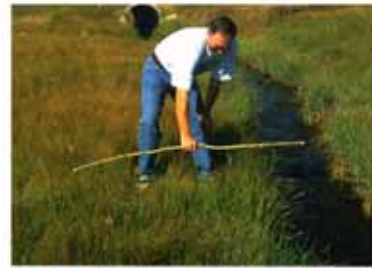
Figure 15—Placement of the measuring pole such that the left end does not reach beyond the center of a stream less than 6 feet wide.
