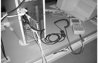
The picture to the left shows how the ProXRS is connected to the computer.
