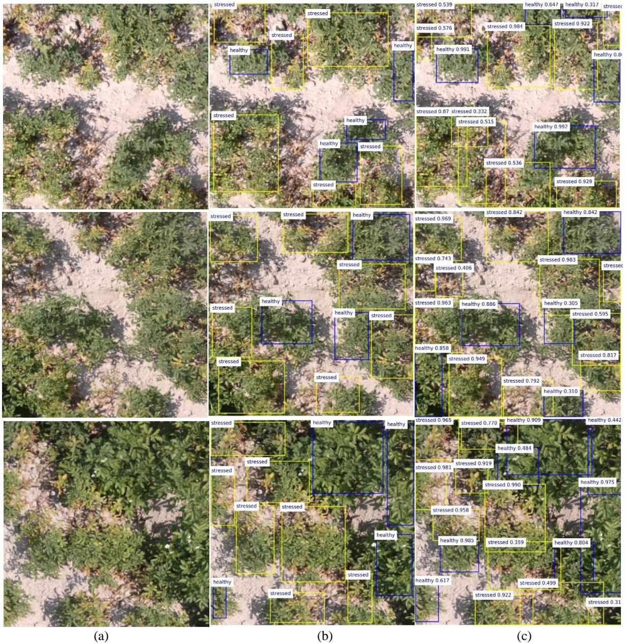
**Figure 4.** (a) Left column: original RGB images from the test set; (b) Middle column: ground truth; (c) Right column: Retina-UNet-Ag predictions showing the object class and level of confidence.
