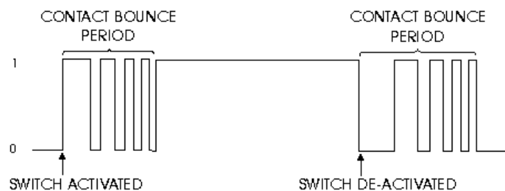
Figure 6. Ideal voltage plot of an active high push button operation showing the results of contact bounce
