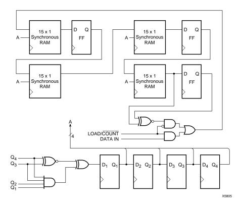
Figure 5: 63-Bit LFSR Counter in 4 CLBs
